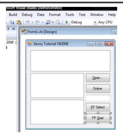
2 Make button event handler function. If user clicks "Open" button, communication setting dialog box of SavoyHsms will appear on the screen. And then establish connection, if user clicks "Open" button. Since communication setting would be saved in "Savoy.ini" file, user doesn't have to change the setting next time.
