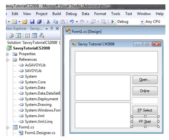
**2** Make button event handler function. If user clicks "Open" button, communication setting dialog box of SavoyHsms will appear on the screen. And then establish connection, if user clicks "Open" button. Since communication setting would be saved in "Savoy.ini" file, user doesn't have to change the setting next time.
